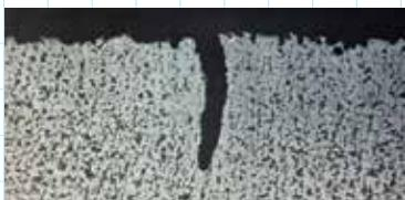
The light area (ferrite) surrounding the dark intrusion is decarburization. Note the lack of pearlite in this decarburized (lighter) zone. There is no evidence of scale, indicating that this defect was created during, rather than prior to rolling.
