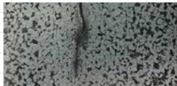
The gray material adjacent to defect within the white decarburized area is subscale. This subscale is evidence that the crack was present on the bloom prior to reheat for rolling.
