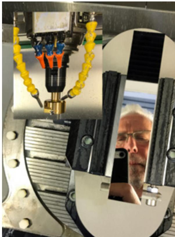
*The mirror finish on this mono-crystalline diamond-milled part is as much a reflection of the machinist’s leadership of the process as it is about the tools.*
