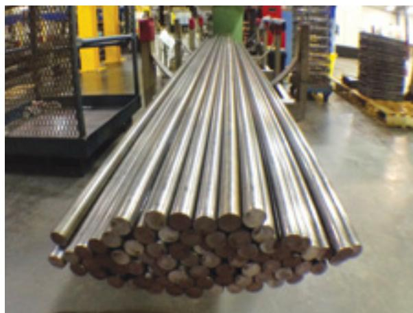
depending on whether it was ordered over 15 feet or less, and whether or not it is thermally treated, could be delivered with straightness of either  $\frac{3}{16}$  inch in 10 feet or  $\frac{1}{16}$  inch in 10 feet. You would never be able to run at commercial production speeds with the hot roll straightness tolerance of  $\frac{1}{4}$  inch in 5 feet!
