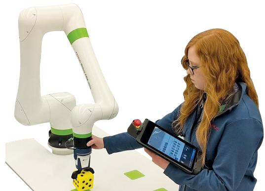
An operator teaches the CRX Collaborative Robot by guiding it manually.
